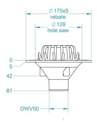
Aquaknight Roof Drains are supplied configurable as either a drain or an overflow
