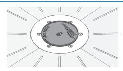
2. Tighten Clamp Ring Screws in a Wheel-Nut sequence in 3 stages: 1) 1Nm, 2) 1.5Nm, 3) 2Nm... firm but not over-tight. Tightening screws further **WILL VOID WARRANTY.** Install Dust Cap.
