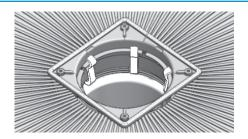
5. Install Clips into sub-tile drainage ports.
