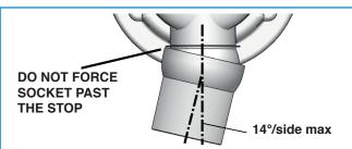
The Swivel Socket rotates 14°/side & downwards. **Do not force the socket past the factory fitted stop** as this may compromise the integrity of the fitting.
