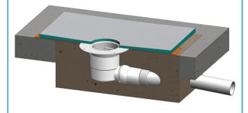
Approved Waterproof Membrane must be detailed down into the throat of Liquid Membrane Flange to the top of Threads
