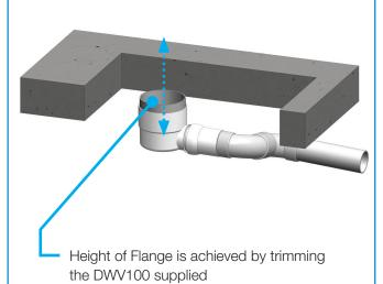
Install Liquid Membrane Flange & set location, height & levels by adjustment of swivel socket
