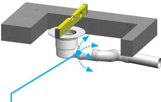
Final position & level of Flange is achieved by adjustment of Swivel Outlet
