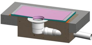
Screw down the Tiling Flange Assembly to finished Tile Height -1mm
