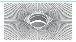
**4**. Screw in Tiling Flange to required height to match Tile thickness. Tiles should sit flush with the top face of Tiling Flange when installed.
