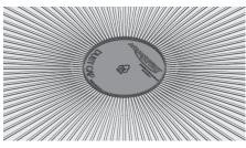
**3**. Apply Thin Set up to edge of Dust Cap radiating out from the centre of waste. Take care to work Thin Set into Clamp Ring Screw heads and remove any trapped air. Remove Dust Cap.
