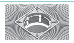
5. Install Clips into sub-tile drainage ports.
