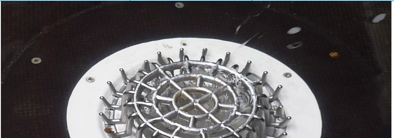
Maximum Weir Flow 480 l/m @ 87 mm HEAD
