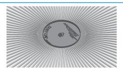
3. Apply Thin Set up to edge of Dust Cap radiating out from the centre of waste. Take care to work Thin Set into Clamp Ring Screw heads and remove any trapped air. Remove Dust Cap.
