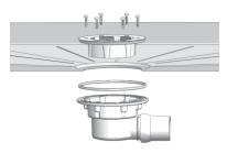
1. Fit Body Assembly to underside of Tile Tray making sure Fixture Seal is seated correctly. Fit Clamp Ring to top side of tray & hand tighten. Check Fixture Seal is properly positioned on the underside of Tile Tray before tightening further.
