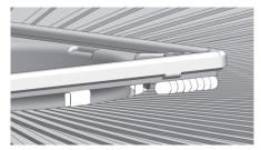
ENSURE THIN-SET DOES NOT ENTER SUB-TILE DRAINAGE PORTS (OBSCURED)
