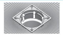
5. Install Clips into sub-tile drainage ports.
