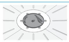
2. Tighten Clamp Ring Screws in a Wheel-Nut sequence in 3 stages: 1)2Nm, 2)6Nm, 3)10Nm... firm but not over-tight. Tightening screws further WILL VOID WARRANTY. Install Dust Cap.
