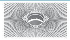
4. Screw in Tiling Flange to required height to match Tile thickness. Tiles should sit flush with the top face of Tiling Flange when installed.
