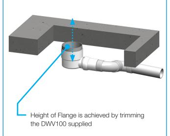
Install Liquid Membrane Flange & set location, height & levels by adjustment of swivel socket
