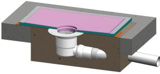
Screw down the Tiling Flange Assembly to finished Tile Height -1mm
