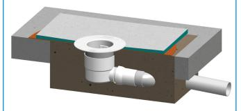
Approved Waterproof Membrane must be detailed down into the throat of Liquid Membrane Flange to the top of Threads
