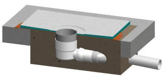
Install Liquid Membrane Flange into DWV100 and seal to Pre-Formed Taper Board
